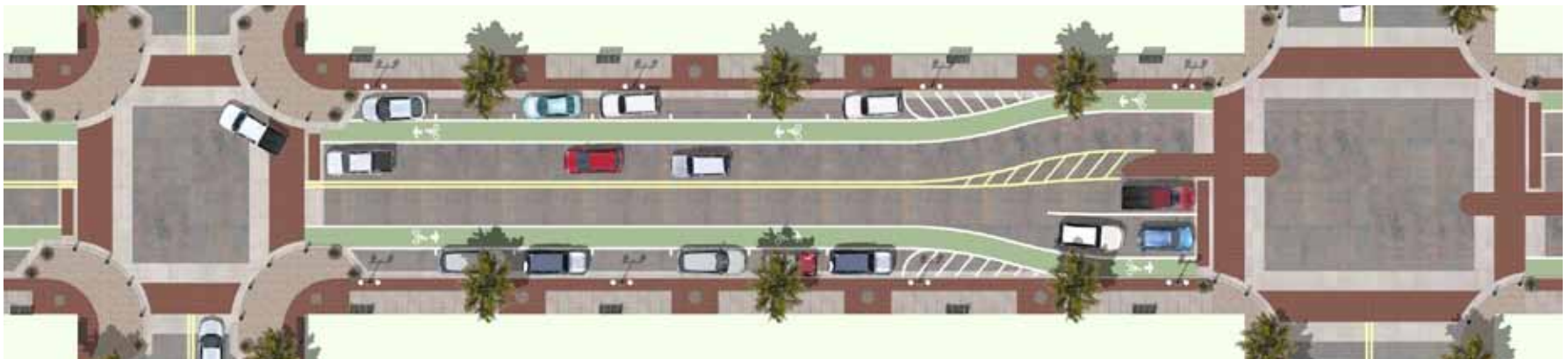
↓ North Avenue Plan View. Right-hand intersection, at 60th and 68th Streets, provides a protected left-turn lane and a surface median refuge for pedestrians. Left-hand intersection is typical, and includes a four-way stop at 64th and 72nd. ↑ North Avenue Perspective. View looks west from 60th or 68th Street intersection.
